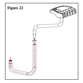
3. Install the unit to sidebox by inserting the arm to the mounting hole on the bottom of sidebox. Then fix the arm with a clip and fasten the clip with a M5\*16 Philip's pan head screw.
