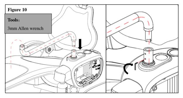
2. Remove the dentist unit after the Delivery head turn around, with the Allen screw in one M6 \* 20 Delivery head and balance arm fixed, prevent rotation.
