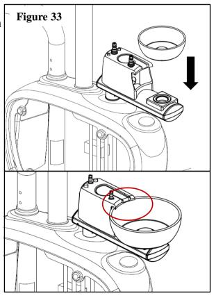
3. Mount the cup filling nozzle, the bowl rinsing nozzle, the drian cup and the cap as the figure shown.
