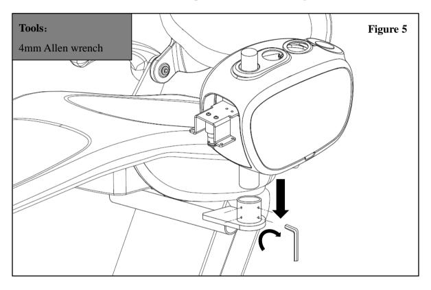
2. Check the levelness of the water unit through a leveling instrument, change the levelness by adjusting the screws on the post.
