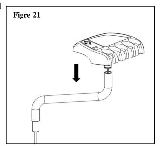
2. Pull the guide rope to make the wire pass through the cosmetic ring and the lower assistant arm. Then joint the two parts of assitant arm together.
