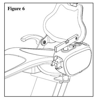
Mount the water bottle cover to the bracket with four M5\*12 outer hex Philips srews.
