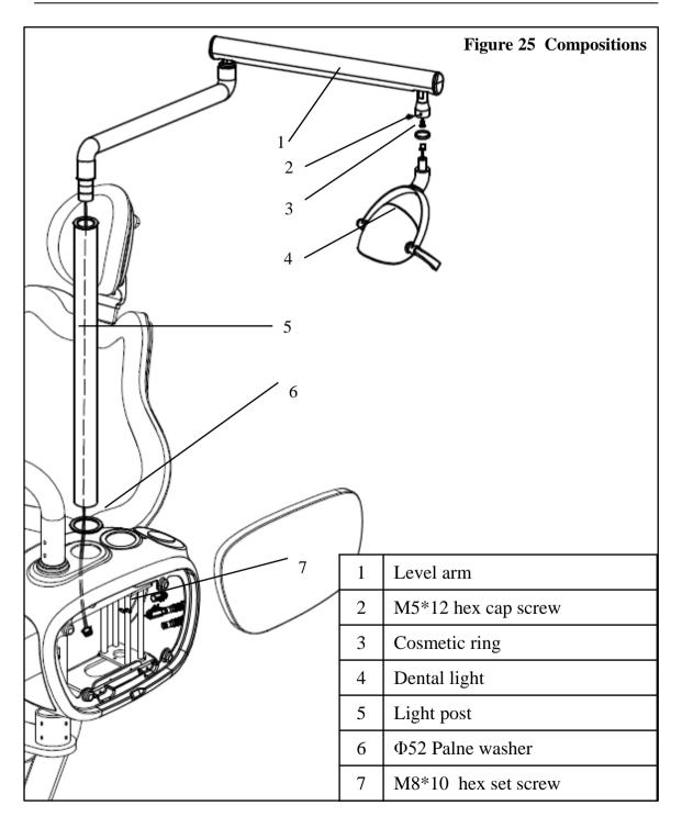
Pass the light post through the palne washer and insert the post into the mounting hole, the end of the post should protrude from the mounting base. Then fix the post with four M8\*10 hex set screws.
