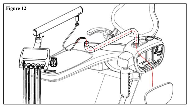
4. Joint the level arm and the rotary arm with three M6\*8 set screws,tighten the screws in clockwise.
