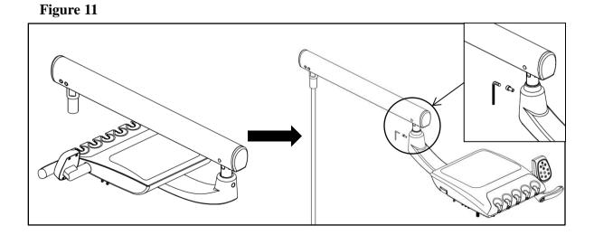
3. Pass the tubes of dentist unit through the cosmetic ring ,tie the tubes with the guide rope, then pull the guide rope and let the tubes route through the rotary arm and approach to the wter unit interior. Joint the level arm and rotary arm together.
