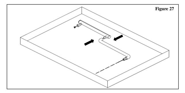
3. Tie up the wire and the guide rope, pull the guide rope to make the wire pass through the post and and approach water unit interior.Then joint the rotary arm and the lght post.
