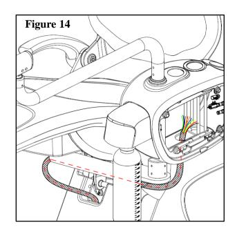
6. The tubes of the dentist unit,the water unit and the reserved should be connected by color.
