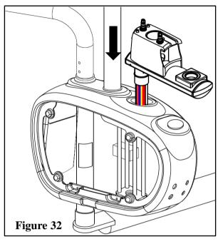
2. Place the cuspidor bowl to its position and fix it on its upper edge.
