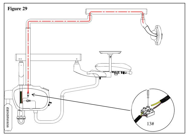
5. Pass the light head shaft through a cosmetic ring and connect the wire terminals , make sure the lamp shaft is well inserted into the level arm, fully fasten with a M5\*12 screw.
